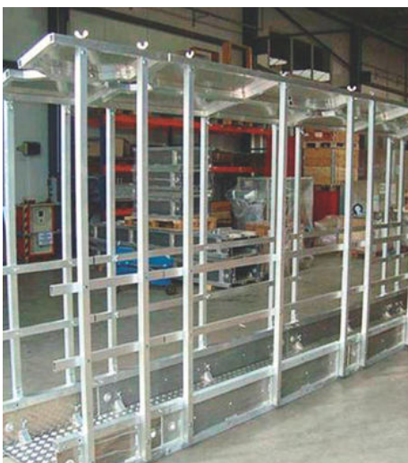
Boiler Stage with Canopy
