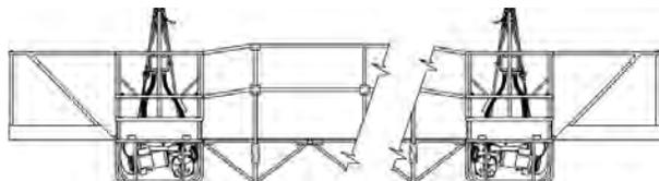
1. When attaching only one fly deck to a swing stage, install the wire rope with the rubber hose under the platform attachment fingers and up through the hole in the toeboard of the Spider.
