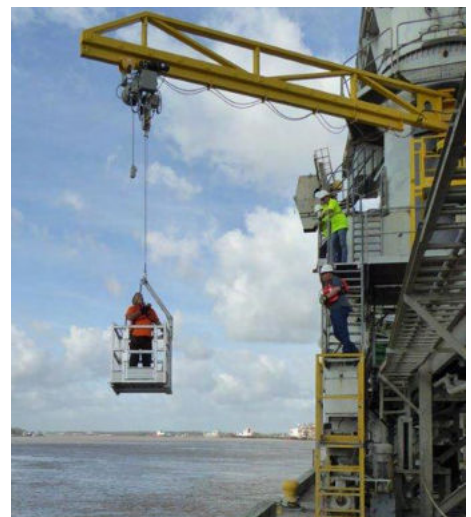
Barge Access System with Powered Trolley
